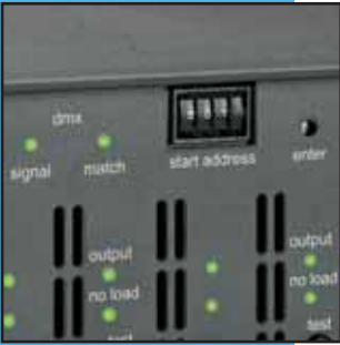
DMX SIGNAL AND DMX SIGNAL MATCH INDICATORS
